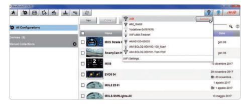
When the PC is authenticated to the network called "AiM" it can see all devices you configured to access the same network. In the image below two AiM devices are connected to the same "AiM" WLAN.
